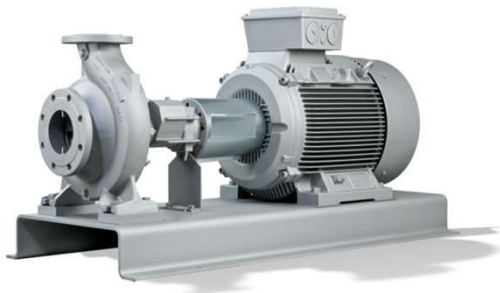
Horizontal Pump (Volute Casing, Mech Seal, Rolling Element Bearings, Oil Lubed)
